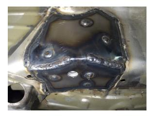
PSD-E46-SUB-004-V2 - QTY.1. - Tailored to fit the NSF Differential Carrier location face/area.
