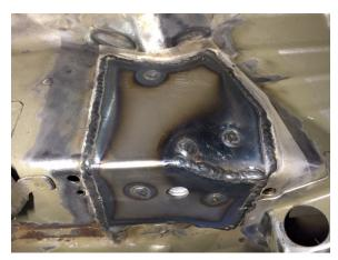
**PSD-E46-SUB-005-V2** - **Qty.2.** - Included in the kit but fitting is optional, they allow the boot floor to be cut from inside the vehicle to gain access to the internal bracing of the subframe to allow welding of the internal features, these plates are used to cap the holes cut in the boot floor. Required for cars built before early 2000.
