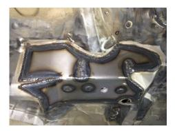
**PSD-E46-SUB-002-V2** – **QTY.1**. – Designed specifically to follow the contours of the OSR subframe Differential carrier location face/area.
