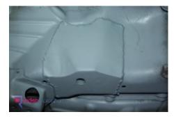
Then an OEM-style seam sealer (spray-applied is the best) over the whole area as well as a heavy seam bead over the weld lines to stop any water or moisture sitting on the plates:
