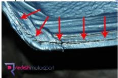
If you found evidence of the 3 or 4 spot welds moving, flexing, or popping (and/or the floor dropping slightly) then clean the seam sealer off and dig it out from between the 2 panels. Stitch weld in 3 or 4 places (below or close to the OEM spot welds) to strengthen and hold the floor to the chassis.
