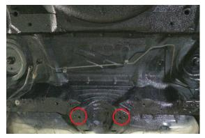
Once the cracks have been weld repaired and the PSDesigns E46 Rear Subframe Reinforcement Plates have been fully welded, use a high build etch primer to coat the bare metal and offer a strong base protection: Notice the horizontal welded join lines and plug welds have been ground smooth.
