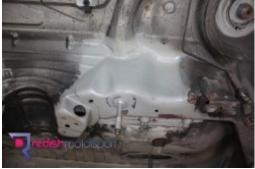
Identify any hairline cracks (if applicable) around the front mounting holes and next to the rear mounting holes. Centre-punch the ends of any hairline cracks <u>BEFORE</u> you take the underseal and factory paint off the floor. Drill 1.5mm 'stop' holes at the ends of any hairline cracks found.
