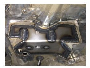
**PSD-E46-SUB-003-V2** - **QTY.1.** - For use at the OSF Differential carrier location face/area. This is the other major problem area on the sub-frame and where cracking is again most common. This plate has been design to dramatically strengthen the OSF location face, spreading the torque loading and unloading over a far greater area, of a stronger material to the original subframe, and repair/cover existing hairline crack(s) or damage.
